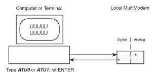
Figure 6-1. Local Analog Loopback Test
